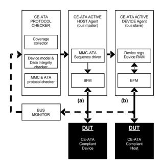
Figure 3: Architecture of the CE-ATA *e* Verification Component (*eVC*)
