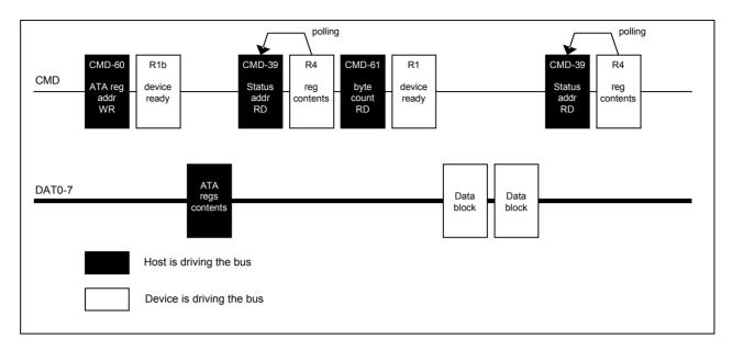
Figure 1: READ\_DMA\_EXT execution over MMC bus.
