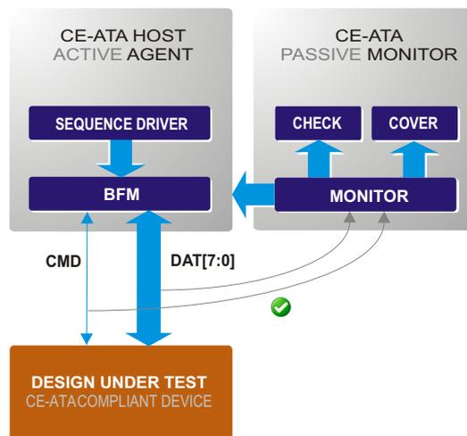
Figure 1: CE-ATA eVC in Host Mode Operation
